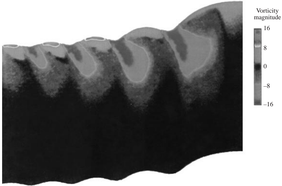
FIGURE 1. Part of the subsurface vorticity field computed numerically by Mui & Dommermuth (1995; their figure 8) for a 5 cm gravity wave. The horizontal distance shown is 2.98 cm. The free surface is plotted with the same vertical and horizontal scale, so that the surface slope is represented correctly. However for the flow beneath the surface, the vertical scale has been dilated; the total vertical extent is only 1 mm.
